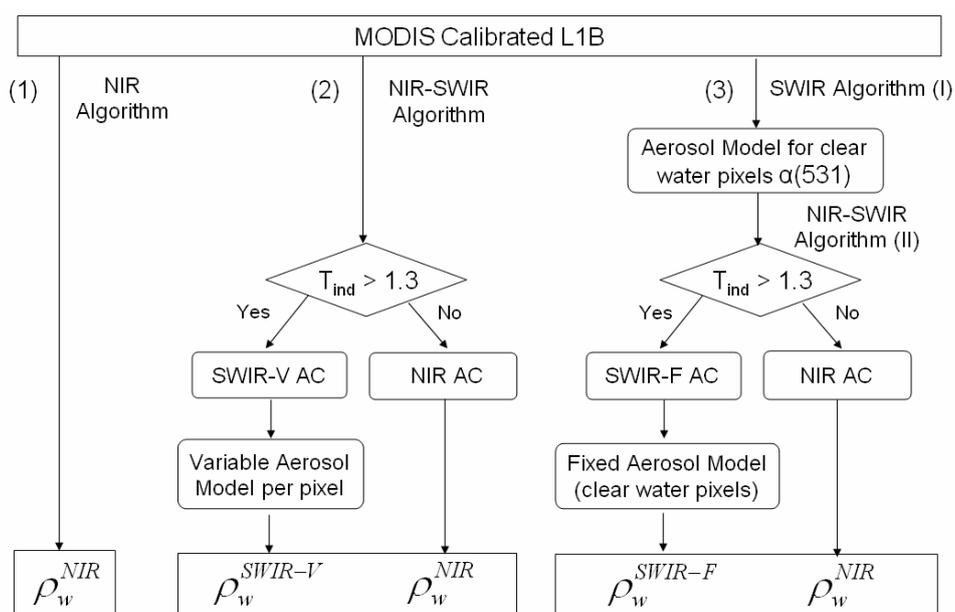
Figure 1. Flow chart of the different atmospheric correction (AC) approaches applied to MODIS-Aqua imagery and analyzed. Reproduced from Dogliotti *et al.* (2011, ONW).
